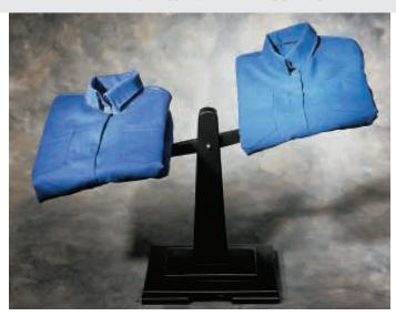
Ultrasoft® FRT Cotton/Nylon Size 44R ASTM F1930 Garment Weight 1.75 lb (796 g) Specified Fabric Weight 7.0 oz/yd² (Actual Fabric Weight 8.1 oz/yd²) Nomex® IIIA Size 44R ASTM F1930 Garment Weight 1.0 lb (457 g) Specified Fabric Weight 4.5 oz/yd² (Actual Fabric Weight 4.7 oz/yd²)
